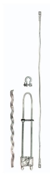
The Fiberlign Deadend is designed to terminate Optical Ground Wire (OPGW) while minimising any compression stresses that may be transferred to the core or optical elements within. The combination of retaining rods, wedge and housing distribute axial and compressive loading over a large area of the OPGW cable. Left-hand or right-hand lay style is provided to suit left-hand or right-hand lay OPGW respectively.
